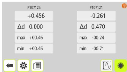
When max min is measured the difference during the measurement is displayed. The max and min values are also displayed.
