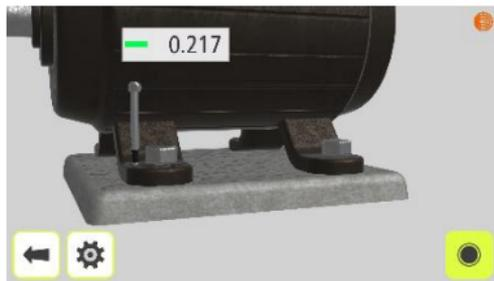
1. Place the Run-Out Probe at the first foot.
