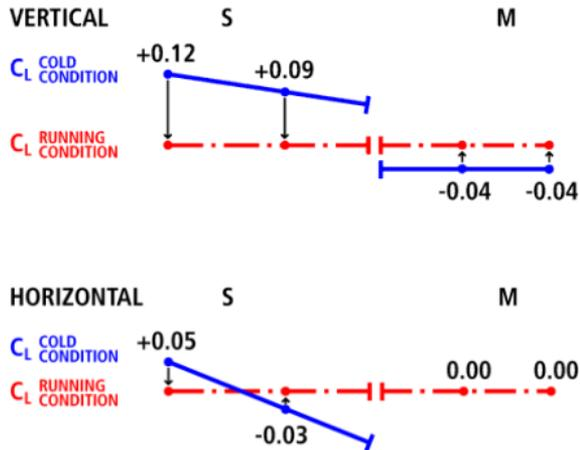
After having entered these feet values, the system calculates how the movable machine should be positioned (target position) in cold condition to obtain perfect alignment during running condition.
