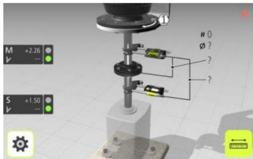
The screen displays the movable machine. The traffic lights show green when the laser hits the detector.
