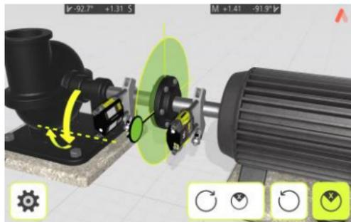
Set the sensors at approximately the same rotational angle at the first measurement position.
