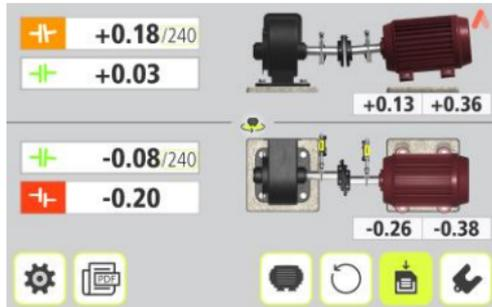
The angular error is shown per coupling diameter.
