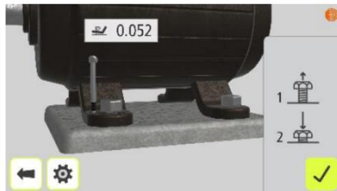
3. Loosen the bolt fully and wait a few seconds.
