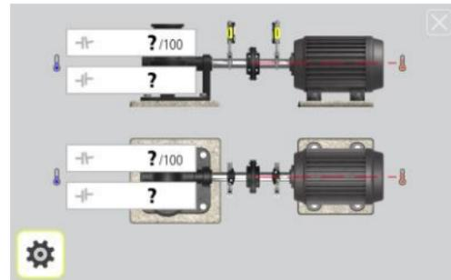
Touch the value boxes and enter target values for the angles in mm/100 mm and target values for the offsets in mm, or mils/inch and mils, according to the pre-set measurement unit.
