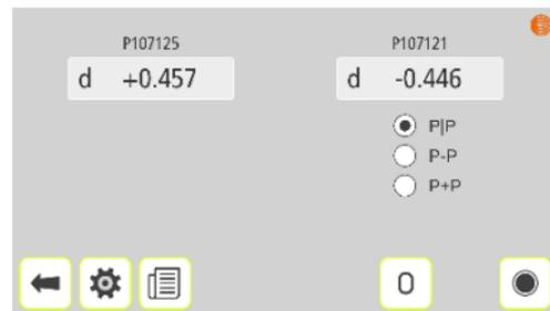
When entering Sensor Display ROP, raw data from the connected Run-Out Probes are displayed.
