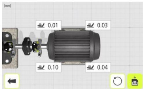
Make the necessary corrections and then check each foot again (the values show approximately how many shims that are needed to eliminate the soft foot).
