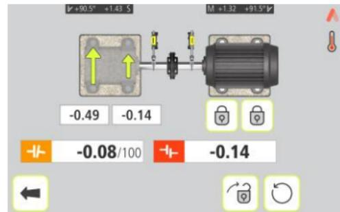
Live values are shown for the two pairs of feet that are not locked.
