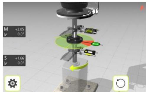
Rotate the shafts to the next position. The shafts must be rotated over a minimum of 45°.
