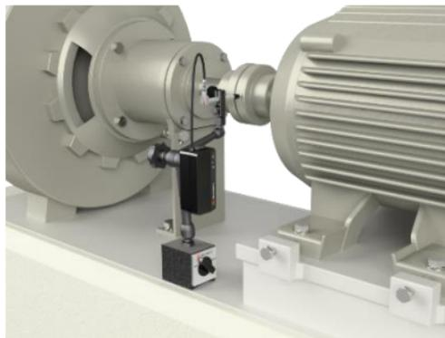
Place the Run-Out Probe on the measurement object.
