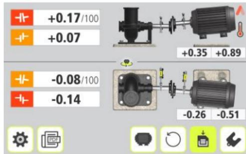
The Measurement Result screen shows coupling values and foot values in both the vertical and horizontal direction.
