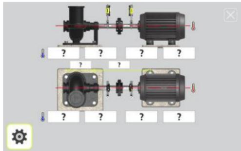
Touch the feet value boxes. Enter target values for the feet in mm or mils according to the pre-set measurement unit together with the required distances.
