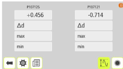
When entering Max Min ROP, raw data from the connected Run-Out Probes are displayed.
