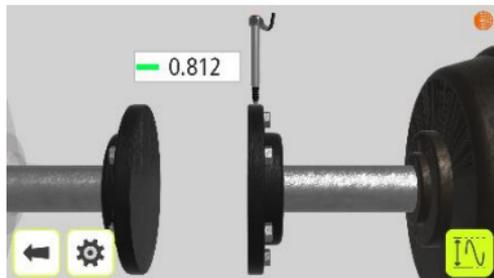
Make sure that the Run-Out Probe is at a suitable part of the measuring range before starting the measurement.
