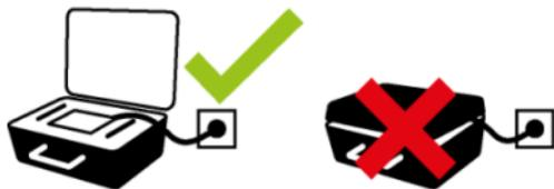
The sensors (M7 and S7) can be connected to their charger and charged while lying in the case. It is important that the lid of the case is open during the charging and that the charger is placed outside the case or else the system will not be charged properly and might be damaged.
