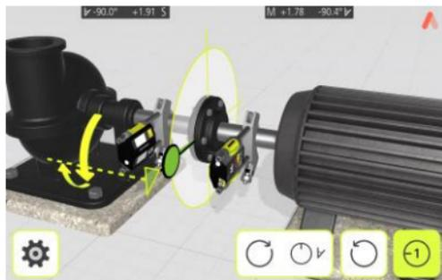
Set the sensors at approximately the same rotational angle at the first measurement position, 9 o'clock.
