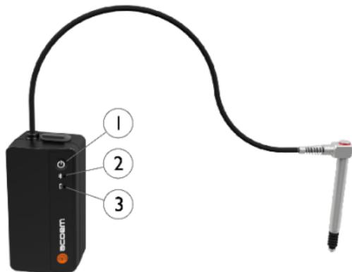
The Run-Out Probe is a battery operated, wireless linear gauge used for measuring run-out on shafts, coupling hubs, flanges and other components used on rotating machinery. It can also be used for distance measurements during adjustments of machinery, soft foot or checks of bearing clearances. The probe is wirelessly connected to the app for registration, display and
