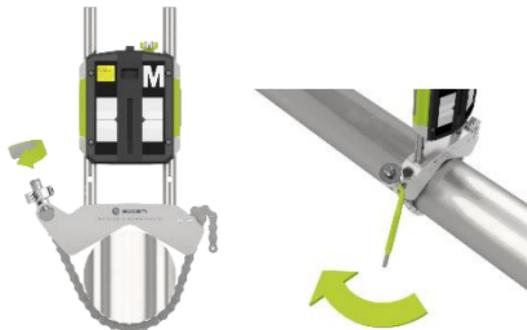
Adjust the height of the sensor by sliding it on the posts until a line of sight is obtained for both lasers. Secure its position by locking both clamping devices on the back of both units.
