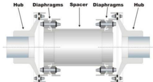
When using the spacer shaft function, the misalignment is presented as an angle for each flexible element. The angles can be compared directly to the figures on allowed misalignment normally delivered from the coupling manufacturer.
