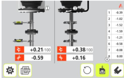
The Measurement Result screen shows coupling values in both directions, and bolt values.
