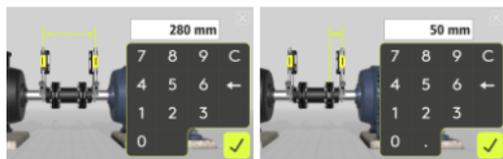
You must enter all the distances. The distance between the sensors, the “spacer shaft length”, the distance between the “end of the spacer shaft” and the M-sensor, the distance between the M-sensor and the first pair of feet and the distance between the first and the second pair of feet.
