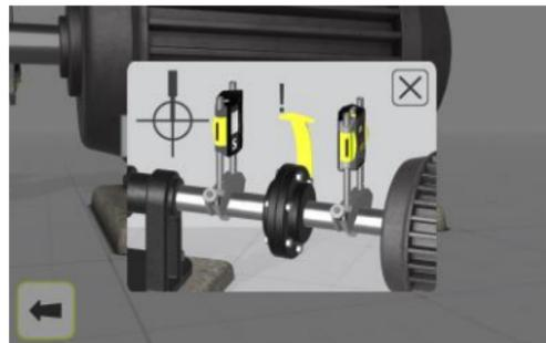
All the distances must be entered, before checking for soft foot.
