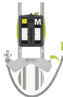
Firmly tighten the chain with the tensioning screw. Use the supplied tensioning tool. Do not over-tighten. If the shaft diameter is too large the chains can be extended with extension chains.
