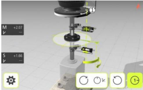
Set the sensors at approximately the same rotational angle at the first measurement position, with bolt number 1 to the right.
