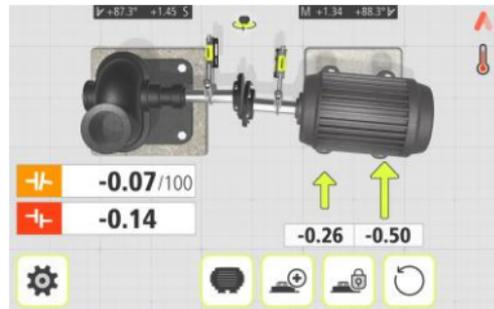
Rotate the shafts to the 3 or 9 o'clock position, if they are not already positioned there. The angle guide helps you to reach the right position.
