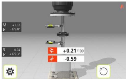
If the angular error has been correctly adjusted in the shimming screen the angular value should now be in tolerance.
