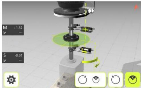
Set the sensors at the first measurement position.
