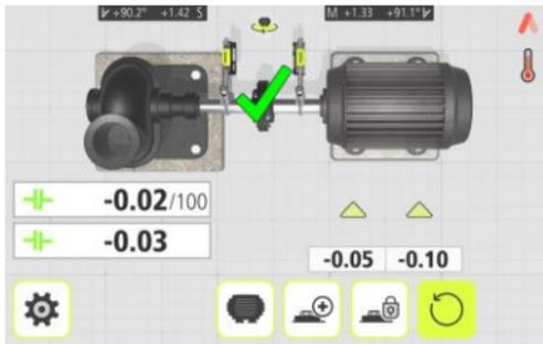
Alignment is now completed. To confirm the result, re-do the measurement.
