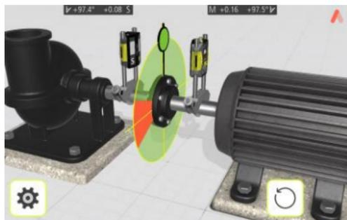
The reading is taken automatically when the sensors have been stationary for 2 seconds.
