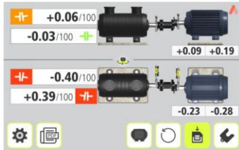
Adjust the machine horizontally until both the angular values are within tolerance. The arrows by the feet show in which direction the machine should be moved.
