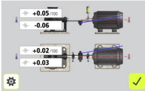
In the example above, the movable machine should be vertically adjusted to a position with an angular misalignment of  $+0.05 \text{ mm}/100 \text{ mm}$  and an offset of  $-0.06 \text{ mm}$ .
