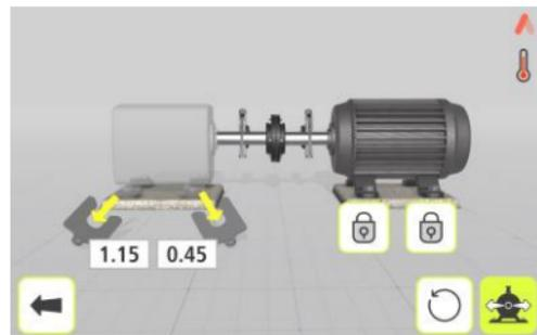
Shim values are shown for the two pairs of feet that are not locked.
