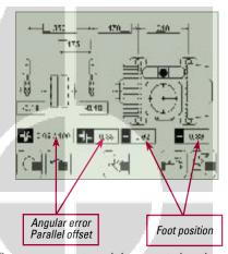
The measurement result is presented on the screen with all relevant information. Angular and offset errors as well as the current foot positions of the movable machine are displayed.
