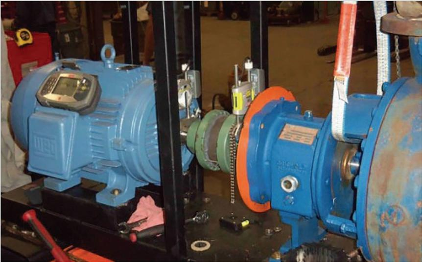
I performed a quick pre-alignment, mounted the equipment and took a reading. The motor needed to come down over 200 mils and move horizontally 406 mils. I wasn't expecting that. So we took another set of readings with the same results. A quick look at the coupling did not show it being off this much.
