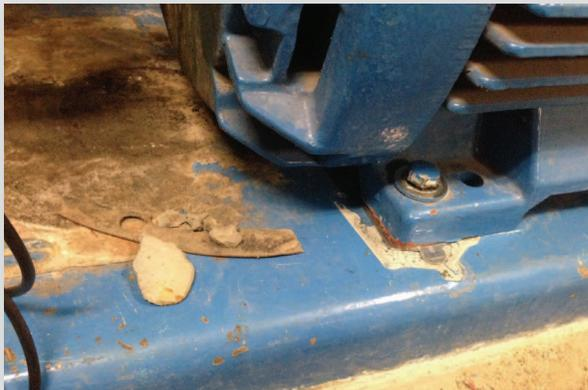
After almost an hour of chiseling, we had the motor sitting flat on all four feet and we were able to proceed with our precision alignment.
