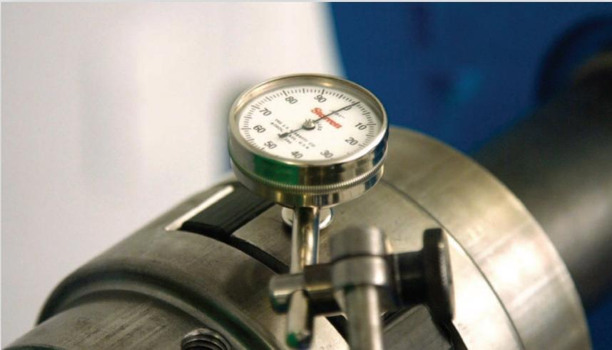
Use a dial indicator and magnetic base. Zero the indicator on the outside diameter of the coupling hub. Slowly rotate the shaft to look for runout, and measure the amount.
