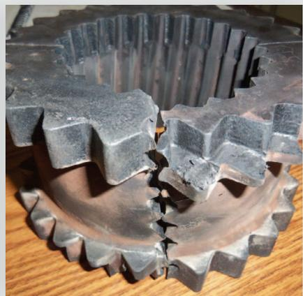
While the couplings did transfer power for a brief time, the loads from misalignment, along with frequent starts, caused them to fail before their time. It's not the coupling's fault. It is a lack of understanding of the differences between coupling misalignment and shaft misalignment. And the coupling, seals, bearings, and productivity pay the price.
