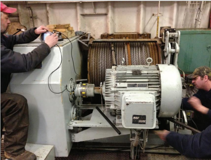
The class wanted to rotate both shafts to perform the alignments, so to take the alignment measurements, we momentarily disengaged the winch drum from the gearbox, rotated the gearbox and motor shafts to each measuring position and then re-engaged the drum to take the alignment measurements. We could have treated this as a
