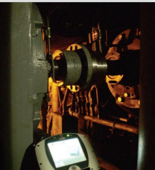
The obvious soft foot check revealed the left rear and right front corners of the motor feet to have 0.025" of angular soft foot, on the outboard side of the motor feet, which was corrected accordingly. The final soft foot correction took an additional 0.005" under the right foot of the motor.
