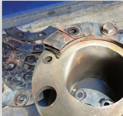
Disc type couplings are fairly “rigid” flexible couplings that can influence the rotational centerlines of each machine, so the class performed the shaft alignment uncoupled.
