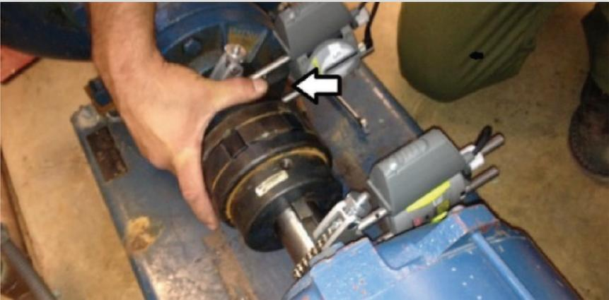
By using this procedure you will minimize the effects of coupling backlash and increase your measurement accuracy! You will end up getting a precision shaft alignment done faster with less moves.
