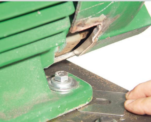
Once the machine has been properly locked out, before loosening any foot bolts, do a quick soft foot check of the feet of both the stationary and the movable components. Using a 0.005" shim or feeler gauge, try to insert the shim under the component feet. Measure for soft foot at three corners of each foot, if three corners are accessible.
