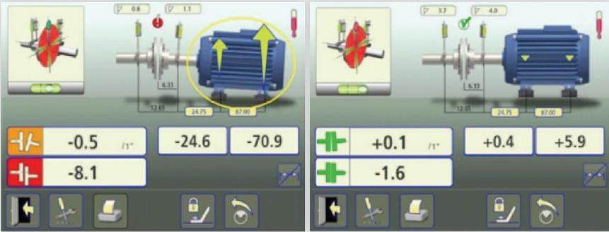
If further minor adjustments are required to meet the vertical and/or horizontal tolerances, do so accordingly; however, remember the sensors need to be in the plane you are correcting as both the vertical and horizontal corrections are done live with adjustable chocks. Once the alignment meets tolerance, document it by saving.
