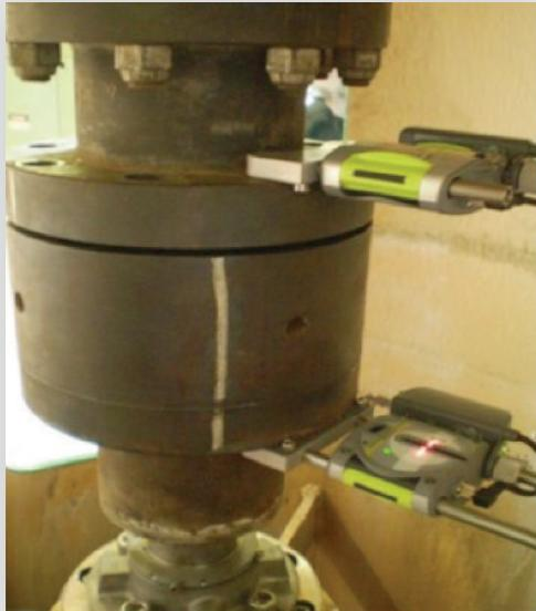
For 1200 rpm, the allowable angular misalignment is  $\pm 1.0$  mil/1" with an allowable offset of  $\pm 6.0$  mils at the coupling center. The initial alignment results revealed the offset misalignment (as viewed from 90 deg. to the #1 bolt) was out of tolerance. The other coupling values were within tolerance.
