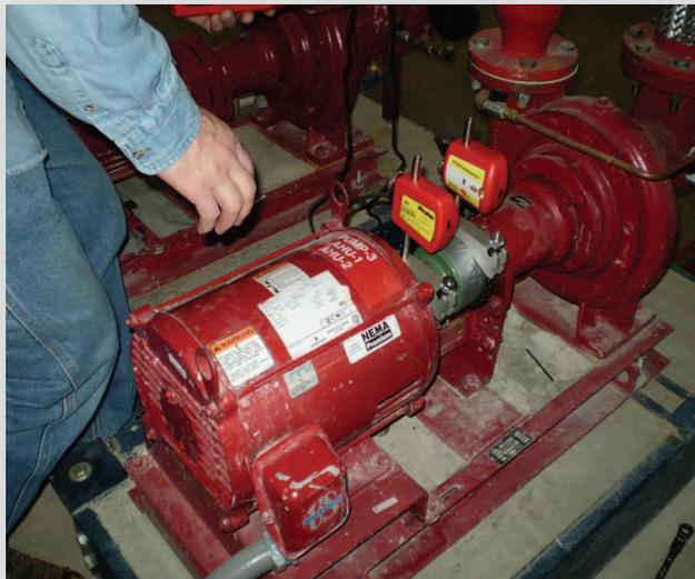
During an alignment of a 10 HP motor/pump set during a training class the vertical alignment corrected easily. However, the horizontal alignment was extremely "sensitive" and would not stay in tolerance
