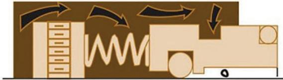
**Figure 3: Non-Pusher Mechanical Seal**
