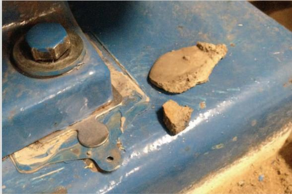
After tilting the motor to the side, we were able to use a hammer and chisel to remove the cement chunks and shims that were stuck by paint to the base.
