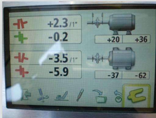
As the motor was moved horizontally the angular coupling value came into tolerance; however the offset coupling tolerance stopped short at -13 mils. There was freedom of movement with the back feet of the
