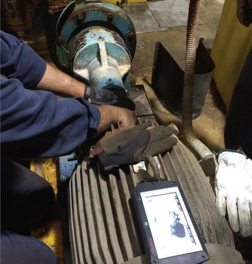
The initial set of alignment results indicated horrible angular misalignment (14 to 16 times tolerance) and offset misalignment (6 to 8 times tolerance) in the vertical and horizontal planes.
