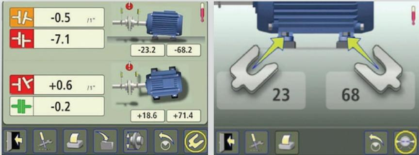
Since the 3rd alignment measurement was taken in the vertical plane, the live screen now shows the vertical view. After the hold down bolts are loosened note, if any, the change in the foot values as you will need to compensate the “live” vertical adjustment by this amount. (Remember the true vertical position of the movable machine is with the hold down bolts tight).
