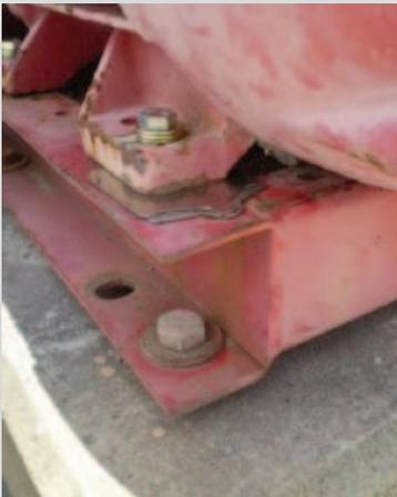
After replacing the hold down bolts and washers the horizontal offset remained spot on as the electric motor feet bolts were tightened.
