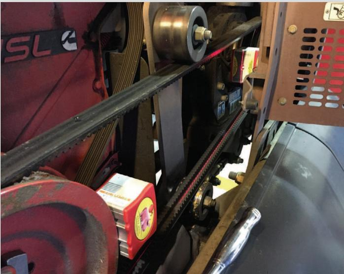
The Belt Hog is used to align the pulleys that drive the AC Screw Compressor.
