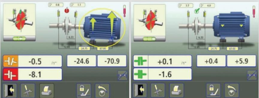
Rotate the shafts to a horizontal plane following the same direction of rotation the alignment measurements were taken in. The XA's screen will automatically change to the horizontal view. Correct the horizontal misalignment, then tighten the hold bolts in a cross torque pattern in three passes. Then re-measure.
