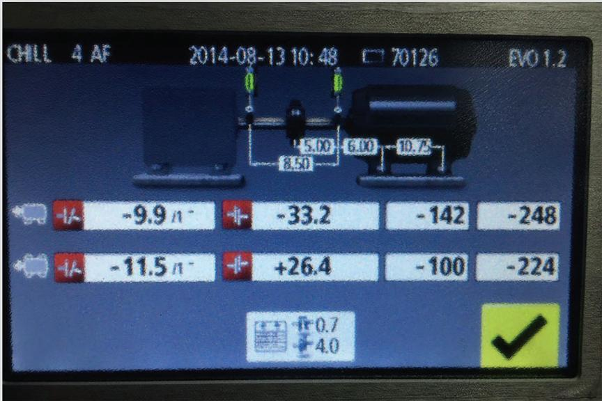
Before making corrections, pre-alignment checks were done which included consolidating the shim stacks under each foot, performing soft foot checks which revealed a 10 mil soft foot on the right front foot that was corrected.
