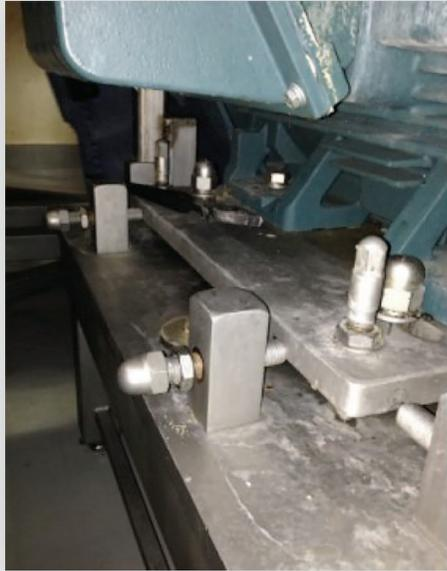
After completing the remaining Pre-alignment steps, we set up the Fixturlaser EVO alignment system, selected the 3600 RPM tolerance and measured the motor shaft condition.
