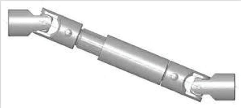
There are two parts that must be understood, proper phasing and angularity of the input and output shafts.
