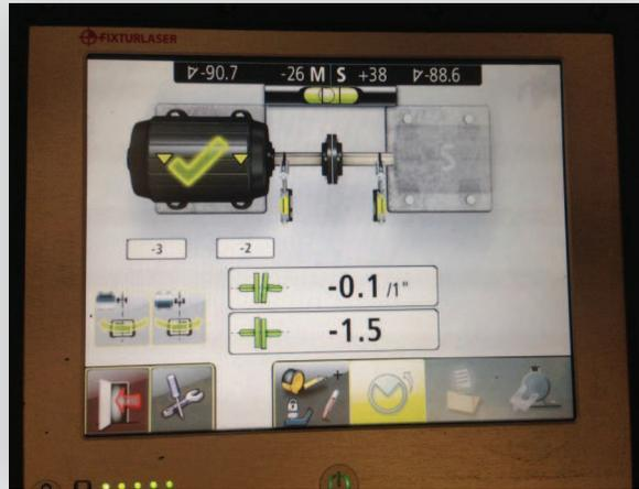
When performing precision laser shaft alignment, part of the pre-alignment steps should be inspection of the hold down bolt washers to eliminate a potential alignment headache. Even if the washers are not cupped it's a good idea to replace "thin" washers with thicker double stacked washers to prevent the thin flat washers from possibly cupping during the shaft alignment you are about to complete.
