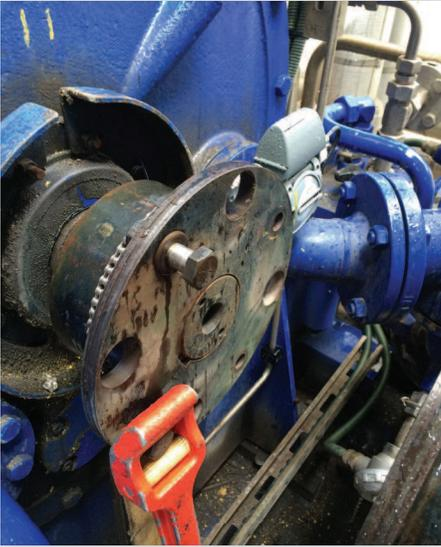
Second, if one of the uncoupled machines turns freely, just the weight of the sensor can cause the shaft to turn when the sensors are in a horizontal plane. You can use a steady rest to rest the sensor against or counterbalance the weight of the sensor to keep the shaft from turning. In this case the mechanics simply hung the strap wrench on a bolt threaded in the coupling hub opposite the sensor.
