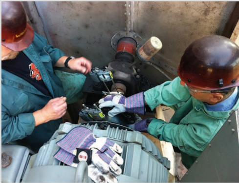
During a recent training class at an Ohio steel mill, we went out to check the alignment on a blower fan that had been experiencing higher than wanted vibration. The shaft alignment was acceptable, but it was noticed that the jacking bolts had been left tight against the motor. The VibrAlign trainer recommended measuring the vibration, then backing off the jacking bolts, and rechecking.
