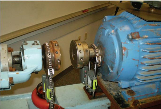
When comparing the “coupled” measurement to the “uncoupled” measurement it is obvious the coupled set isn’t close to the true vertical position of the motor to the pump as indicated by the uncoupled set. In this case the flexible coupling and gross misalignment, together, are influencing the Vertical Angle by 1.5mils/1”, the Vertical Offset by 17 mils, the front foot by 31 mils, and the rear foot by 47 mils!
