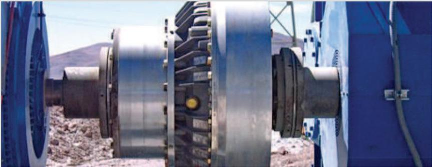
This conveyor is one of two side-by-side conveyors; each is 60" wide by 500 yards long. The gearbox has a backstop which only allows a clockwise rotation as viewed from the rear of the electric motor. The other conveyor was in operation during the alignment.
