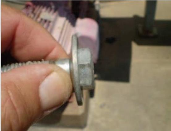
The electric motor feet had fairly large bolt holes with soft steel washers under the hold down bolts. As the motor feet were tightened, the cupped washers "centered" the motor feet holes causing the horizontal offset to change and move out of tolerance.
