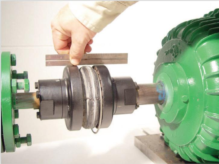
Using a straightedge, check the tops of the coupling flanges for parallelism. If a gap exists while checking for parallelism, measure the gap with a shim, or feeler gauge. Insert the measured amount of shim under each of the movable machines to bring the components into rough vertical alignment. Repeat the procedure on the sides of the coupling flanges to correct for rough horizontal alignment. Be sure to tighten the feet of the movable machine back down before beginning alignment.
