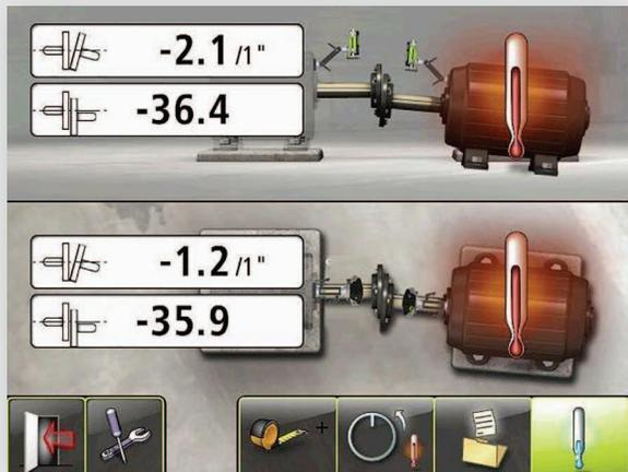
3rd – After allowing the machines to cool to ambient temperature take the cold readings and save it. The “Cold” position will be displayed. Note: This is not an indication of the actual cold alignment, but simply a known “Cold” Position.
