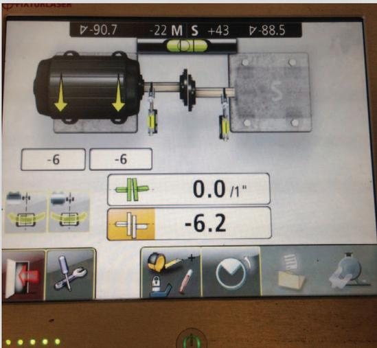
The cupped washers were pulling our motor 6 mils to the side, moving it out of the horizontal offset tolerance as indicated by the Orange Coupling Icon.
