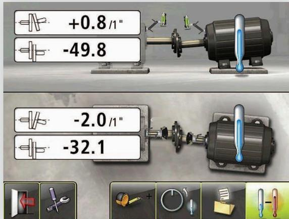
4th – Once these measurements have been saved, the NXA will compare the Cold minus Hot readings and display the REAL Targets needed to compensate for dynamic changes from Offline 2 Running. The Targets are then saved for
