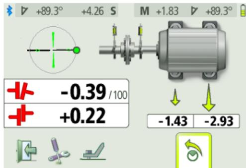
Rotate the shafts to the 3 or 9 o'clock position to make adjustments in the horizontal direction. The angle guide helps you to reach the right position.
