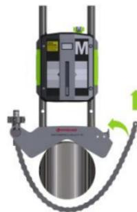
Firmly tighten the chain with the tensioning screw. If necessary, use the supplied tensioning tool. Do not over-tighten. If the shaft diameter is too large the chains can be extended with extension chains.
