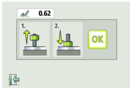
Loosen the bolt fully and then tighten it firmly, preferably with a dynamometric wrench.
