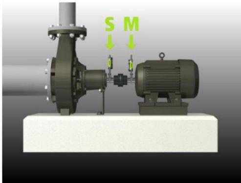
After rotating the shafts into different measuring positions the system calculates the relative distance between the two shafts in two planes. The distances between the two measuring planes, distance to the coupling and distances to the machine feet are entered into the system. The display box then shows the actual alignment condition together with the position of the feet.
