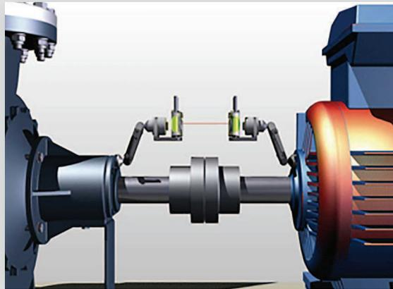
2nd – Take the “Live” hot reading with the machines at full running state, up to temperature and under common load and save it.
