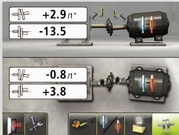
future shaft alignments. At this point you can align the machine as indicated by the procedure. Simply touch the coupling icon and align the machine. You will now have a true precision shaft alignment.
