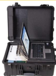
ONEPROD VMS transportable case 16 or 32 channels with BNC connectors (Available with different functionality levels and with or without PC)
