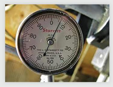
So, if a straight edge isn't sufficient for precision machinery, what about dial indicators?
