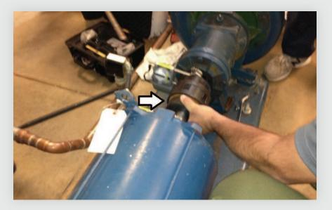
Then move the sensors to 11 o'clock keeping the coupling engaged from the motor side. Take the second measurement.
