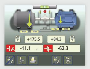
After the horizontal correction was made and hold down bolts tightened, a new set of measurements was taken followed by a slight vertical and horizontal adjustment. A final measurement was
