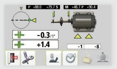
Lastly, we evaluated our vertical alignment figures to assure there was no unintended movement. Once confident in the alignment condition, we torqued the jam nuts utilizing a cross- pattern tightening sequence and re-measured for final confirmation.
