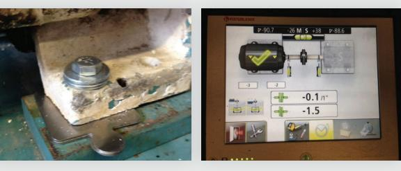
When performing precision laser shaft alignment, part of the prealignment steps should be inspection of the hold down bolt washers to eliminate a potential alignment headache. Even if the washers are not cupped it's a good idea to replace "thin" washers with thicker double stacked washers to prevent the thin flat washers from possibly cupping during the shaft alignment you are about to complete.
