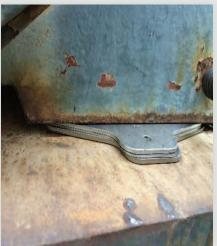
3 shims in this shim stack. Solid footing.
