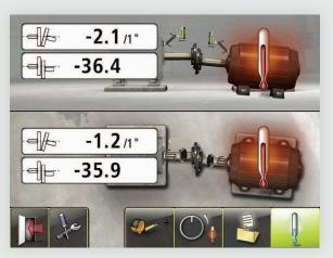
3rd – After allowing the machines to cool to ambient temperature take the cold readings and save it. The "Cold" position will be displayed. Note: This is not an indication of the actual cold alignment, but simply a known "Cold" Position.
