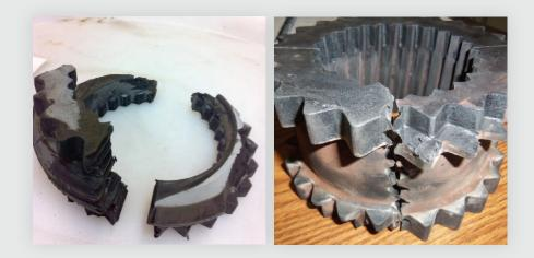
While the couplings did transfer power for a brief time, the loads from misalignment, along with frequent starts, caused them to fail before their time. It's not the coupling's fault. It is a lack of understanding of the differences between coupling misalignment and shaft misalignment. And the coupling, seals, bearings, and productivity pay the price.
