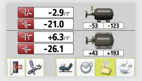
We began the Verti-Zontal correction process and because of the vertical jack bolts, bypassed the shimming screen straight to the live screen. Using the EVO live screen with the sensors in the vertical plane allows you to perform vertical adjustments on this type of machine while simultaneously observing the motor shaft position.
