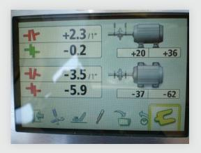
As the motor was moved horizontally the angular coupling value came into tolerance; however the offset coupling tolerance stopped short at -13 mils. There was freedom of movement with the back feet of the motor but the front feet were bolt bound by 10 mils and no adjustment of the motor could get the offset misalignment in tolerance.
