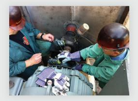
During a recent training class at an Ohio steel mill, we went out to check the alignment on a blower fan that had been experiencing higher than wanted vibration. The shaft alignment was acceptable, but it was noticed that the jacking bolts had been left tight against the motor. The VibrAlign trainer recommended measuring the vibration, then backing off the jacking bolts, and rechecking. The following reductions in vibration (in inches per second) resulted:
