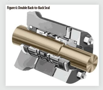
The more common multiple seal configuration is called a Double (dual pressurized) seal, where the two seal face sets are oriented in opposite directions. The features of this seal arrangement are:
