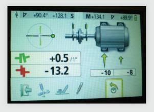
loosen the pump and move the coupling in the opposite direction the display screen shows we need to move the motor." He was correct.
