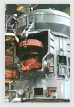
Bowl mills are used to pulverize coal prior to being blown into coal-fired boilers. They are very large machines with heavy rotating components usually driven by an internal planetary gear set in the bottom of the mill. A typical steam generation power plant will have multiple bowl mills for each boiler in the facility.
