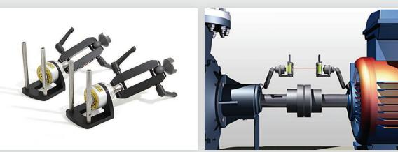
2nd – Take the "Live" hot reading with the machines at full running state, up to temperat<u>ure and under common load and save it.</u>
