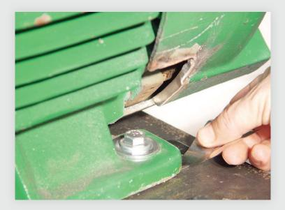
Be mindful of an angular soft foot. If a movable machine foot has an angular soft foot, you may have to cut a partial shim or shims to correct for angular soft foot.
