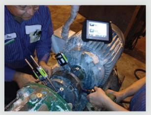
The first go around they seemed very confident and went about the alignment seemingly without issue. They removed all the old shims, cleaned under the feet, corrected soft foot, took alignment readings, made the exact
