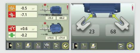
Since the 3rd alignment measurement was taken in the vertical plane, the live screen now shows the vertical view. After the hold down bolts are loosened note, if any, the change in the foot values as you will need to compensate the "live" vertical adjustment by this amount. (Remember the true vertical position of the movable machine is with the hold down bolts tight).
