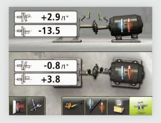
future shaft alignments. At this point you can align the machine as indicated by the procedure. Simply touch the coupling icon and align the machine. You will now have a true precision shaft alignment. This is a much-abbreviated explanation of the OL2R process. With training and practice this process can yield very positive results for your company or customers.
