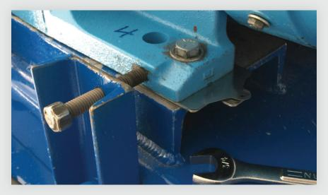
One thing is certain, DO NOT directly hit the motor or machine foot! This means don't use a hammer or brass bar to hit the foot or machine directly. If the only means to move a machine is this type of force, use an intermediary device to soften the blow. Otherwise, direct consequences will occur that may not be immediately evident.
