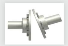
• Vertical/horizontal offset misalignment, where the shafts are parallel vertically/horizontally, but not collinear, or in the same line.
