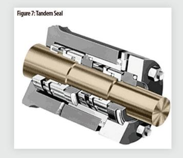
The other multiple seal configuration is called a Tandem (dual unpressurized) arrangement, where the two individual seals are positioned in the same direction. This seal arrangement is commonly used in Submersible wastewater pumps, between the pump and motor, with oil as the barrier liquid. The typical features of this seal arrangement are:
