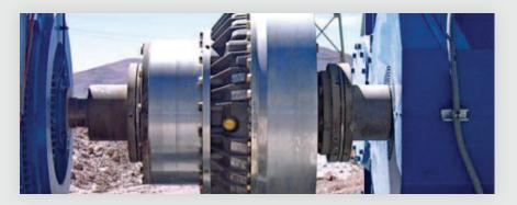
This conveyor is one of two side-by-side conveyors; each is 60" wide by 500 yards long. The gearbox has a backstop which only allows a clockwise rotation as viewed from the rear of the electric motor. The other conveyor was in operation during the alignment.
