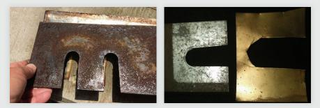
You should take the time to wire wheel the base and feet to clean out any dirt, rust, or debris and always use clean shims with no bent edges or fold lines.
