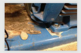
After almost an hour of chiseling, we had the motor sitting flat on all four feet and we were able to proceed with our precision alignment.
