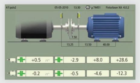
A second set of alignment measurements were taken with final results of:
