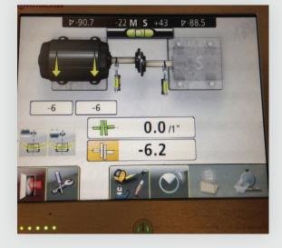
The cupped washers were pulling our motor 6 mils to the side, moving it out of the horizontal offset tolerance as indicated by the Orange Coupling Icon. We replaced all the washers at each motor foot with 2 thicker washers and the problem was solved. Our alignment came right in at better than the 3600 RPM tolerances of +/- 0.5mil/1" angularity and +/- 2.0 mil offset.
