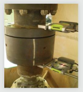
measurements are then registered with the sensors first pointed at the #1 bolt, second at 90 deg. and third 180 deg. from the #1 bolt.
