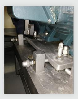
motor feet was not possible due to an obstruction blocking the right side motor feet. Challenged by this barrier, we decided the vertical jack bolts were a viable alternative for making vertical corrections.
