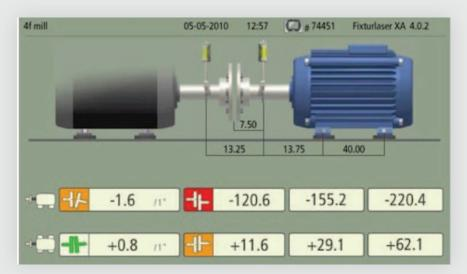
The first set of alignment measurements were taken with initial results of:
