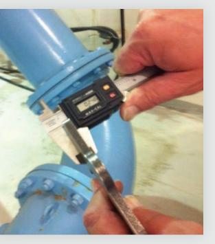
We also checked each shim in several locations to make sure the thickness was uniform. If the shim had more than a 2 mil variation. we would discard it. The reason is we have a 2 mil soft foot tolerance and would not want to create an angular soft foot because of shim quality. We also would recommend that you mic all shims 50 mils and thicker. The thicker the shim. the more likely there are variations. We have seen 125 mil shims as thin as 114 mils. 11 mils thinner.
