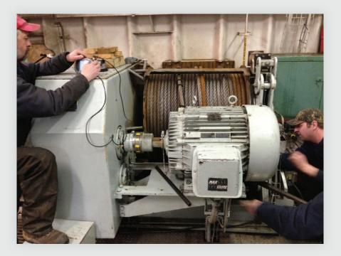
The class wanted to rotate both shafts to perform the alignments, so to take the alignment measurements, we momentarily disengaged the winch drum from the gearbox, rotated the gearbox and motor shafts to each measuring position and then re-engaged the drum to take the alignment measurements. We could have treated this as a non-rotating shaft alignment and broken the coupling loose to do so. However more accurate misalignment data is obtained when both shafts are rotated.
