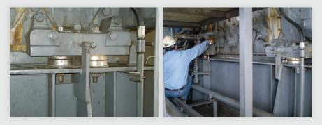
The Verti-Zontal process is modified slightly by taking the three alignment measurements from top to bottom (12 o'clock, 3 o'clock and 6 o'clock, for example) vs. side to side (9 o'clock, 12 o'clock and 3 o'clock) as when aligning a "shimmed" machine. After the results are analyzed press the shim icon as you normally would and note the feet position. This is the vertical position of the movable machine at the feet **BEFORE** the hold down bolts are loosened. Then press the live adjustment icon.
