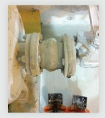
• The shafts had been running about 3/8" out of alignment in the horizontal plane. That's 374 mils of offset misalignment or about 93 times the 4.0 mils maximum allowable offset misalignment for 1800 RPM!
