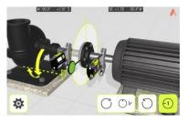
Set the sensors at approximately the same rotational angle at the first measurement position, 9 o'clock.
