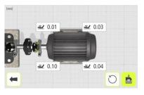
Make the necessary corrections and then check each foot again (the values show approximately how many shims that are needed to eliminate the soft foot).
