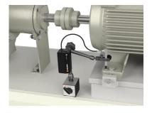
A soft foot condition needs to be corrected before any alignment takes place. If not, the measurement result will be of no value. It is more or less impossible to establish if there is a soft foot condition without using some kind of measurement tool. The Softcheck ROP application checks each foot and displays the result in mm or mils.
