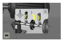
All the distances must be entered, before checking for soft foot.
