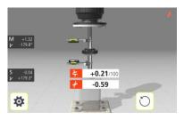
If the angular error has been correctly adjusted in the shimming screen the angular value should now be in tolerance.
