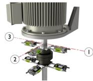
Place yourself at the position corresponding to the second measurement position, where it is easiest to turn the shafts through 180°.
