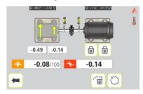
Live values are shown for the two pairs of feet that are not locked.
