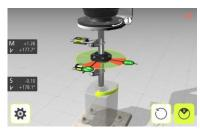
The reading is taken automatically when the sensors have been stationary for 2 seconds.
