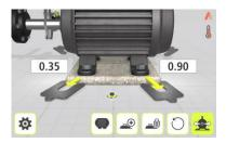
The Shimming screen shows foot values in the vertical direction as suitable shim values (0.05 mm / 1 mil).
