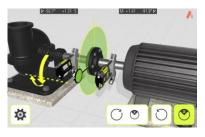
Set the sensors at approximately the same rotational angle at the first measurement position.
