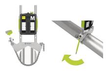
Adjust the height of the sensor by sliding it on the posts until a line of sight is obtained for both lasers. Secure its position by locking both clamping devices on the back of both units.
