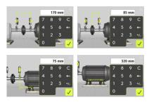
You must enter all the distances. The distance between the sensors, the distance between the center of the coupling and the Msensor, the distance between the Msensor and the first pair of feet and the distance between the first and the second pairs of feet.
