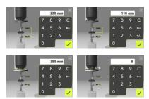
You must enter all the distances. The distance between the sensors, the distance between the center of the coupling and the Msensor, the pitch circle diameter, and the number of bolts.
