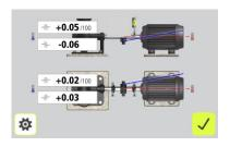
In the example above, the movable machine should be vertically adjusted to a position with an angular misalignment of +0.05 mm/100 mm and an offset of -0.06 mm.
