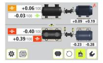
Adjust the machine horizontally until both the angular values are within tolerance. The arrows by the feet show in which direction the machine should be moved.
