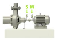
After rotating the shafts into different measuring positions, the system calculates the relative distance between the two shafts in two planes. The distances between the two measuring planes, distance to the coupling and distances to the machine feet are entered into the system. The display box then shows the actual alignment condition together with the position of the feet. Adjustment of the machine can be made directly, according to the displayed values.
