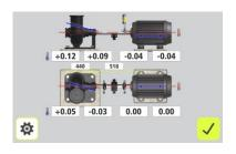
In the example above, the stationary machine will shrink vertically by 0.12 mm at the rear feet and 0.09 mm at front feet while the movable machine will expand 0.04 mm while running.
