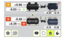
The Measurement Result screen shows coupling values and foot values in both the vertical and horizontal direction.
