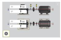
Touch the value boxes and enter target values for the angles in mm/100 mm and target values for the offsets in mm, or mils/inch and mils, according to the pre-set measurement unit.
