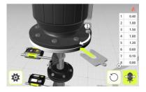
The Shimming screen shows bolt values as suitable shim values (0.05 mm / 1 mil).
