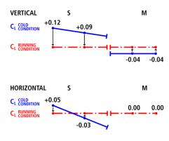
After having entered these feet values, the system calculates how the movable machine should be positioned (target position) in cold condition to obtain perfect alignment during running condition.
