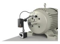
Place the Run-Out Probe on the measurement object.
