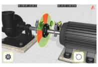
The reading is taken automatically when the sensors have been stationary for 2 seconds.
